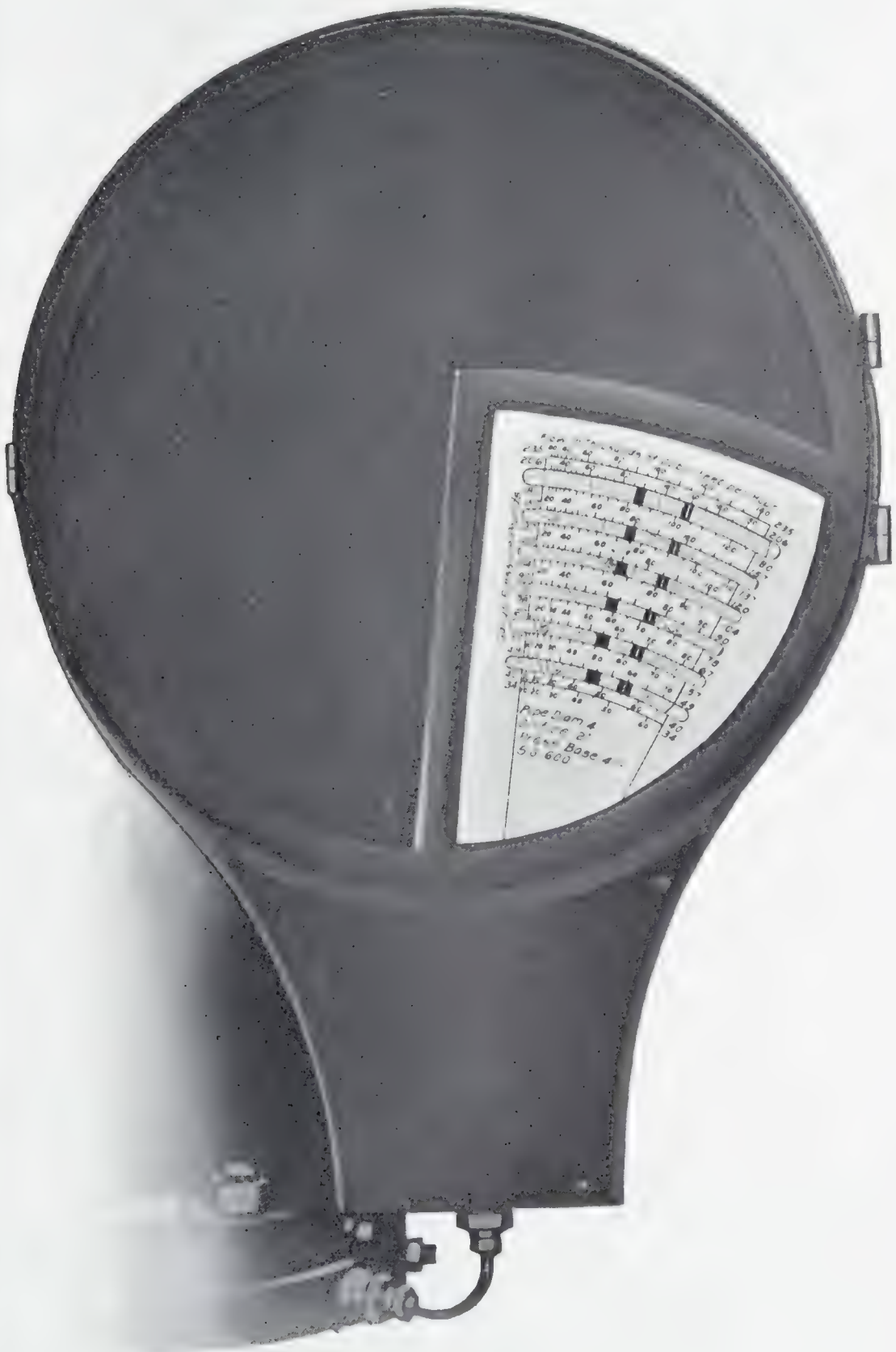
Fig. 119—DIFFERENTIAL GAUGE WHICH INDICATES RATE OF FLOW PER HOUR. SEE PAGES 130 AND 131.
